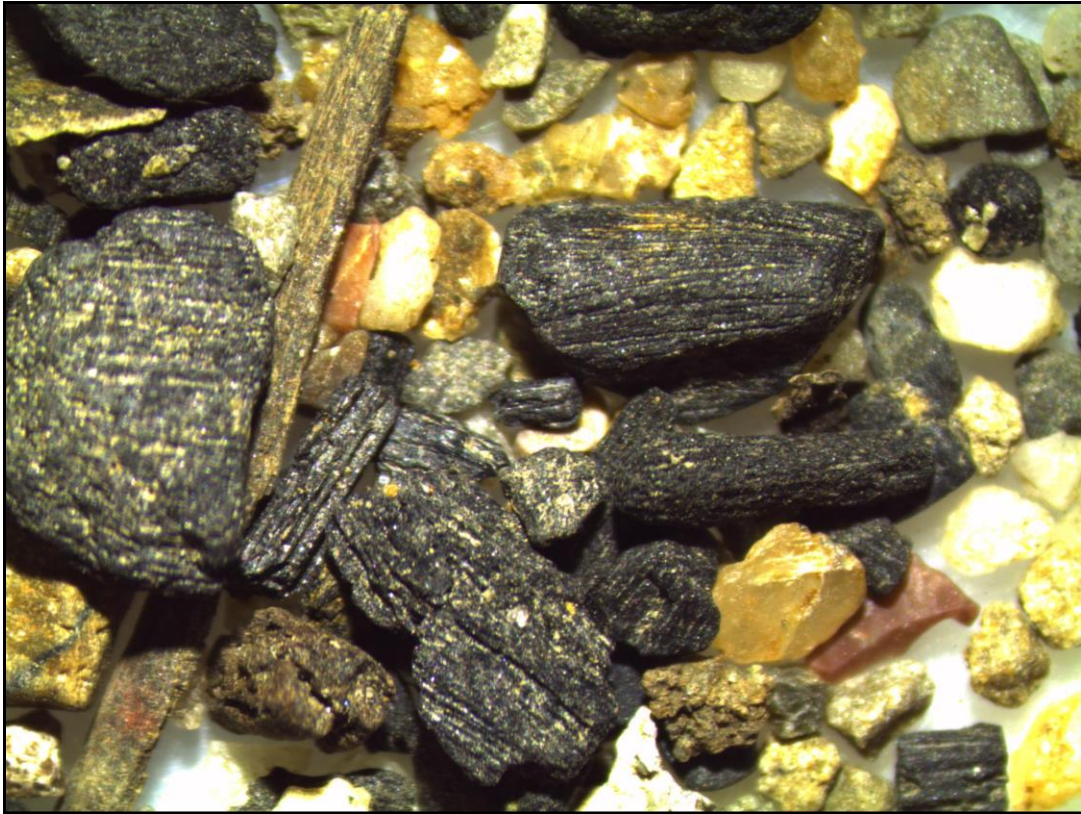
Figure 3: Image of coarse sieve fraction showing abundance of quartz grains and lithic clasts. Note the charcoal fragments and plant matter in this fraction.
