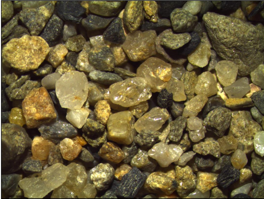
Figure 3: Image of coarse sieve fraction showing abundance of quartz grains and lithic clasts.
