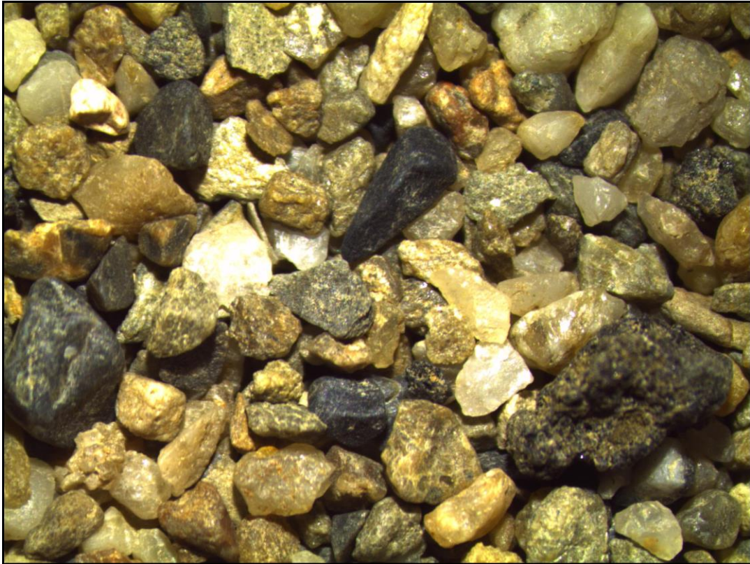
Figure 3: Image of coarse sieve fraction showing common quartz and lithic clasts
